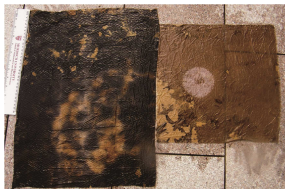
Fig 4. Silk and cotton changed color to black purple (Hue5Y3/2) and yellow brown (Hue10YR4/6-6/6) after one day of dyeing 4 times.
