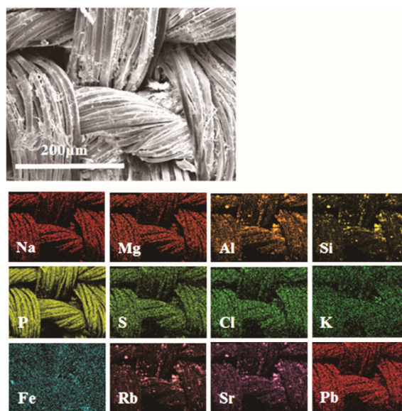
Fig 5. Scanning electron microscopy equipped with energy dispersive analysis (SEM-EDS) of black purple part on silk, showing the spectra and elemental content maps of dyed silk with various elements.
